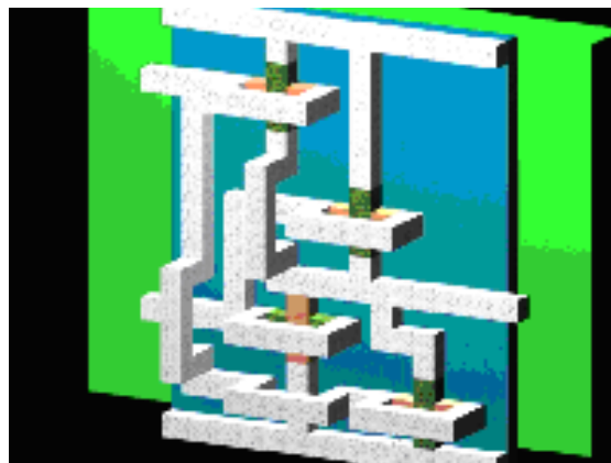
Figure 3. A design for a NAND gate made up of conducting, insulating, p-type, and n-type MBB's.
